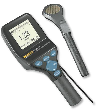
The ASM-990 Series Advanced Survey Meter can detect alpha, beta, gamma, or x-ray radiation within an operating range of 1  $\mu$ R/hr to 1 R/hr (1 to 5,000,000 CPM), depending on the selected probe (Geiger-Mueller, neutron, proportional counter, scintillation). With the proper probe combination, this meter can be used as a general survey meter, an area monitor, a wipe-test counter, and a contamination monitor.
